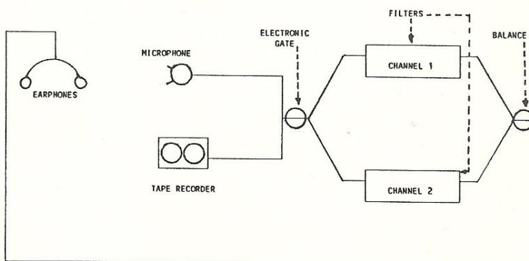
Fig. 2 - Diagram of the Electronic Ear
